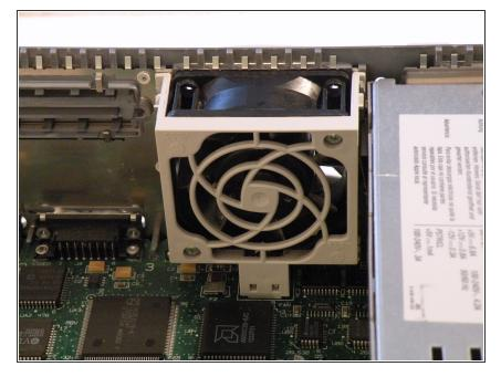
The fan recieves power from two contacts on the logic board and has no connector.
