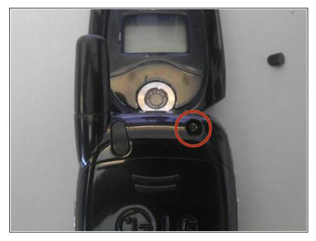
• Remove a single Phillips #00 screw from beneath the cover.
