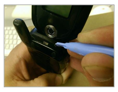
Starting at the seam near the antenna, use a plastic opening tool to gently pry the back plate from the phone.
