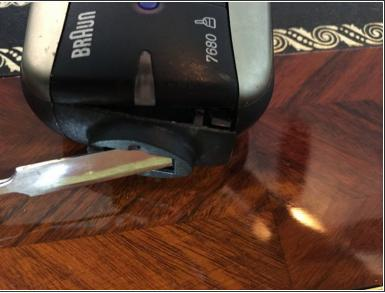
First pry the left side of the cover off, then pry the right side of the cover off before removing. Trying
