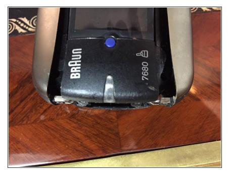
Pull the side covers off from the bottom, they hinge from the top and will come off freely once you rotate them up and away from the body starting at the bottom.
