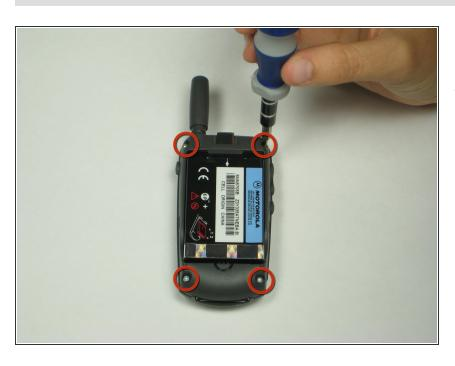
Using a T6 Torx Screwdriver remove the four torxs on the back of the phone.
