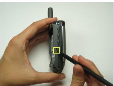
Simultaneously press indicated buttons on both sides of phone.
