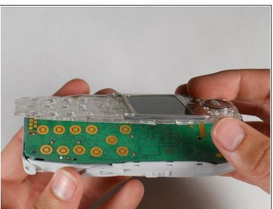
Insert spudger between screen assembly and phone body.
