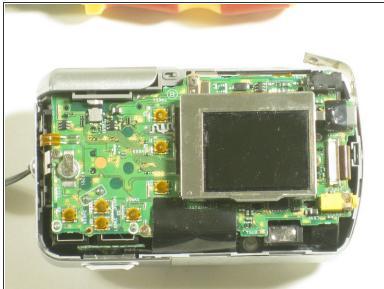
Remove outer case. Pull the back away from the main body of the camera.
