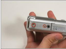
Locate all five screws on the camera. Then proceed to remove all the screws.
