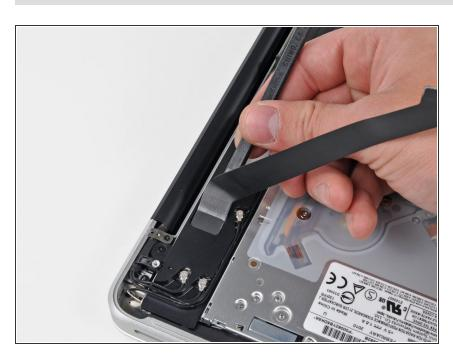
Use the flat end of a spudger to pry the AirPort/Bluetooth cable connector up off its socket on the AirPort/Bluetooth board. To reassemble your device, follow these instructions in reverse order.
