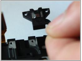
Unscrew the 2.9mm phillips #000 screws from the audio jack and remove component from the tablet.
