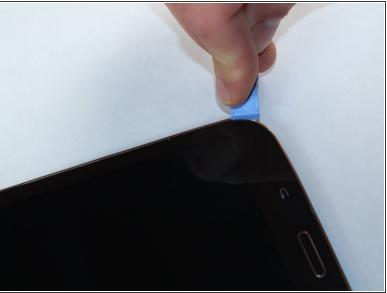
Start out by separating the screen from the back cover using the larger plastic opening tool to pry them apart.
