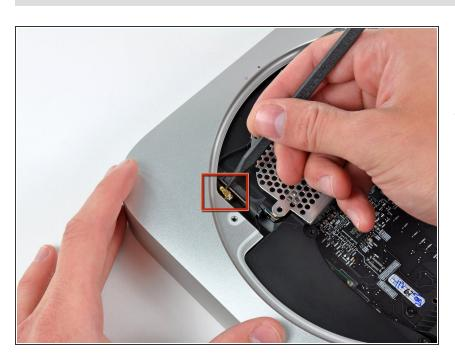
The top Wi-Fi antenna connector is hidden underneath the antenna plate near the hard drive connector.
