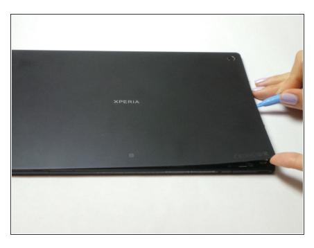
Slide the plastic removal tool along the edges.
