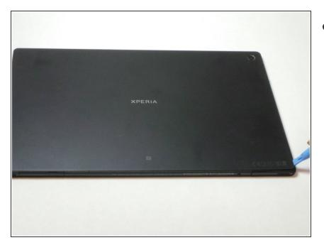
Place the plastic removal tool in the corner of the object.
