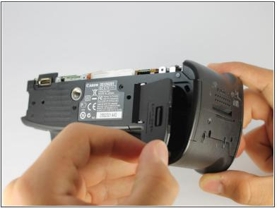
Open the battery flap by pressing the button on the flap in a direction parallel to the bottom of the device while also pulling away from the device.
