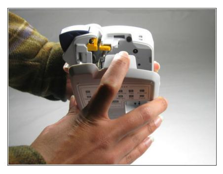
Open the back cover of the device by pressing on the indication arrow and pulling it open.
