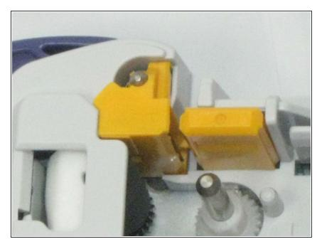
Locate the yellow cutter blade unit as shown in the photo.
