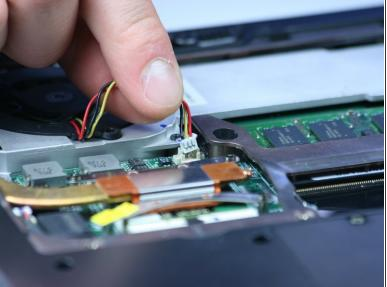
There are red, yellow, and black set of wires going to a white connector. Grab the three cables and pull straight up, away from the computer.
