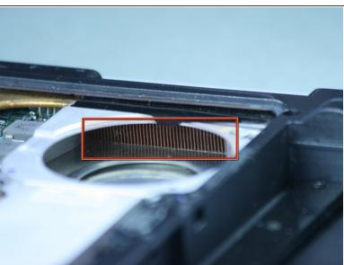
Use a cotton swab to remove dust. Also you can use compressed air, blow air from the inside out to clear dust from vent, or heat sink.
