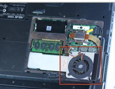
Remove highlighted screws, pry open case at highlighted spot.
