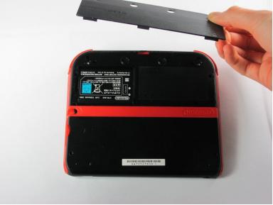
Hinge the upper rear panel upwards and outwards to remove it.
