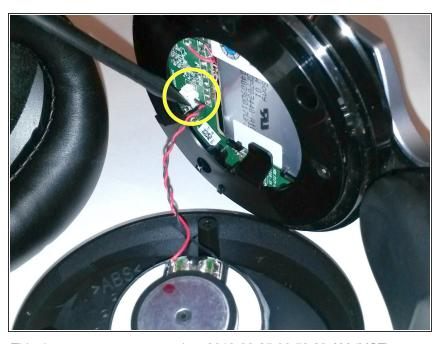
Using tweezers, gently pry the red and black speaker wires from the attached socket.
