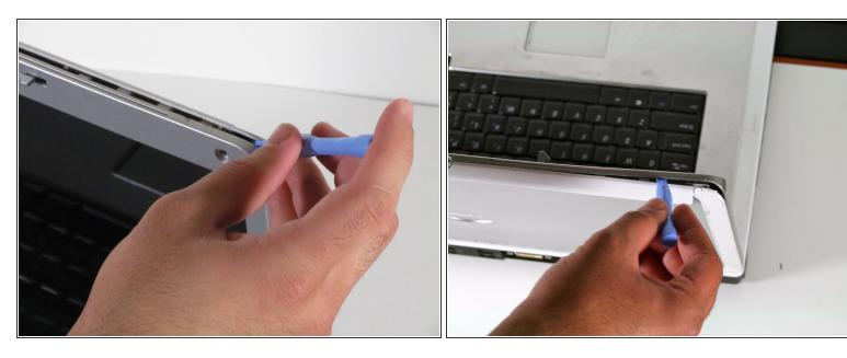
• Use a plastic opening tool to carefully pry the plastic cover from the screen mount.
