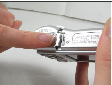
The battery compartment is located on the bottom side of the camera. Push the button in, and slide the cover to get access to the batteries.
