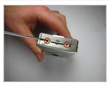
Remove screws on strap panel of camera.
