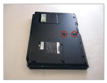
Locate the two clips on the bottom of the computer that support the battery.
