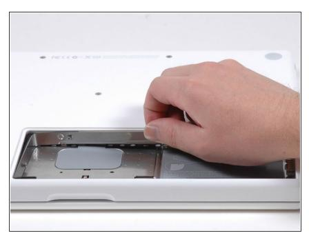
Rotate the L-shaped memory cover so it clears the battery compartment opening and lift it up and out of the computer.
