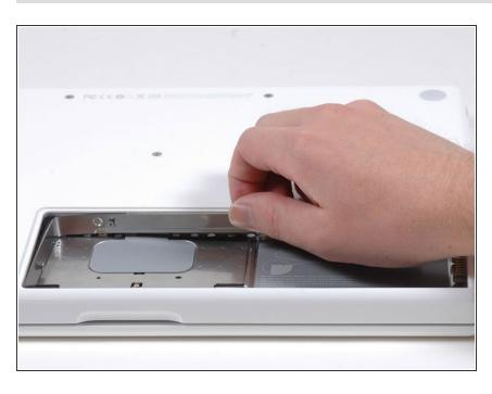
Rotate the L-shaped memory cover so it clears the battery compartment opening and lift it up and out of the computer.
