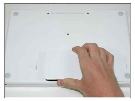
Lift the battery out of the computer.
