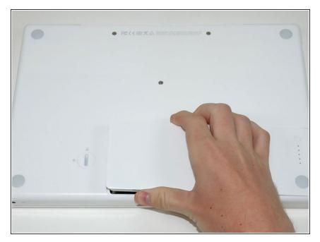
Lift the battery out of the computer.
