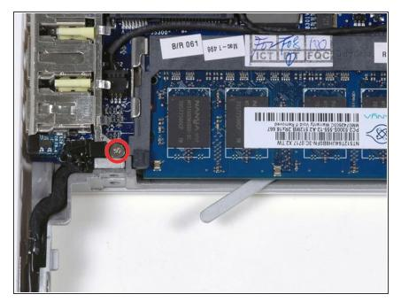
Remove the single Phillips screw near the battery connector.
