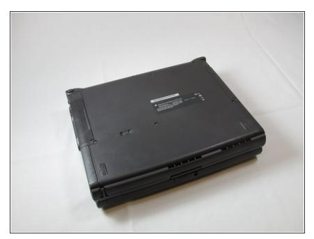
Close the screen and turn the PowerBook over. Orient the computer so the text of the label is right side up.
