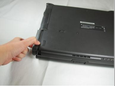
Press and hold the button on the left of the front side, and slide the battery out.
