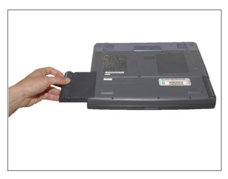
To replace, insert the new floppy disk drive with the wording facing down.
