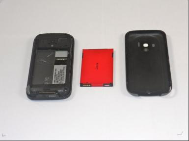
Remove the battery by lifting upward from the slot located on the right hand side.
