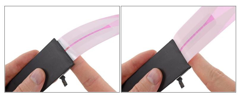
Using your fingertip, gently roll the adhesive strips over the bottom edge of the battery, toward the back.
