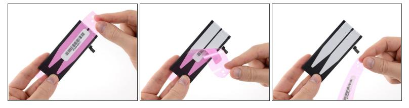
Carefully peel away the remaining piece of film, fully exposing the adhesive strips.
