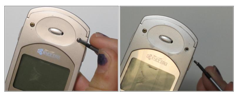
Remove the four tiny front screen screws with a screw driver
