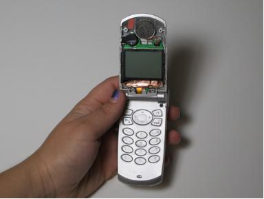
• Carefully remove screen after prying it lose, exposing the bottom screen and parts
