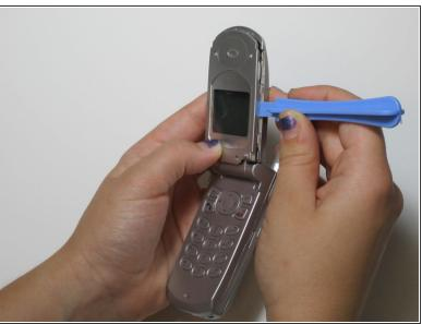
Use prying tool to open the side of the screen and work you way around the screen.
