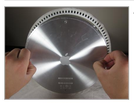
Carefully remove the base access panel.
