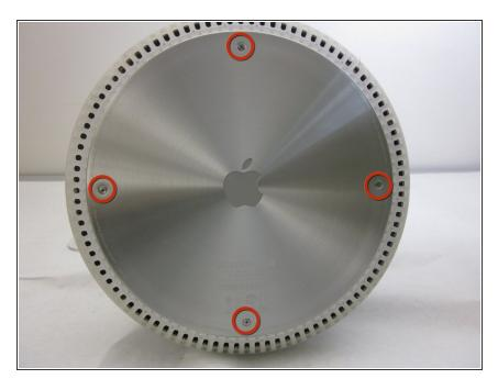
Loosen the four Phillips #0 screws.
