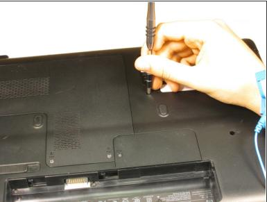
• Remove the 6mm screw above the laptop stickers using a Phillips #0 screwdriver.
