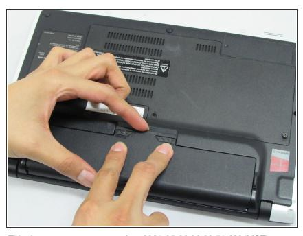
Locate the two latches with the words "lock" and "release" on them.
