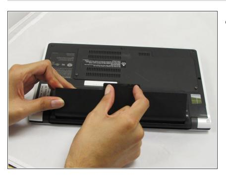
Push the latches towards each other and lift the battery to remove it.
