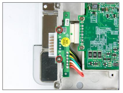
Remove the two Phillips screws securing the battery connector to the metal framework.
