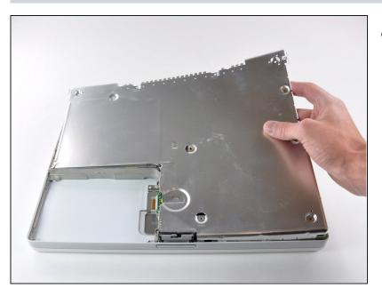
• Lift the bottom shield off.
