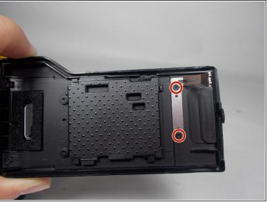
• Once the compartment is open and unscrew the two 0.5mm Phillips screws that hold the spring in place. Replace the spring with a new one.
