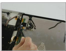
Next, remove the metal shield covering the other ribbon. Then remove the ribbon.
