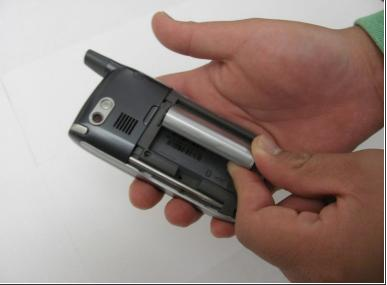
• Use the small notch on the left hand side of the phone to remove the battery.
