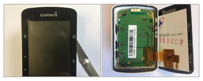
Using the sharp implement, VERY carefully move around the edge of the glass screen and prise the screen up out of the case.
