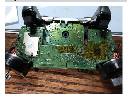
• Remove the 2 Torx (T6) screws.
