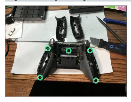
• Remove the 5 Torx Security Bit (TR9) screws.
