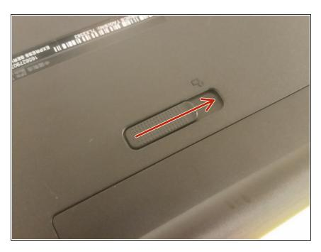
Flip the laptop over, battery facing you. Move the latch to the right, and grab the battery as it comes up.
